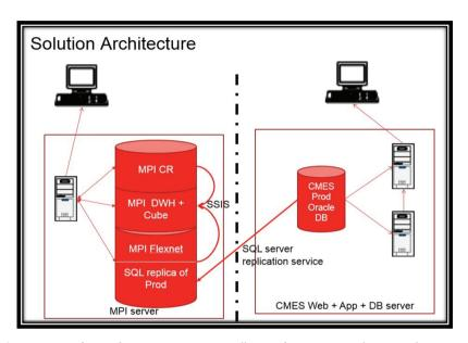
Figure 7: MPI (Manufacturing Process Intelligence) reporting solution architecture.
