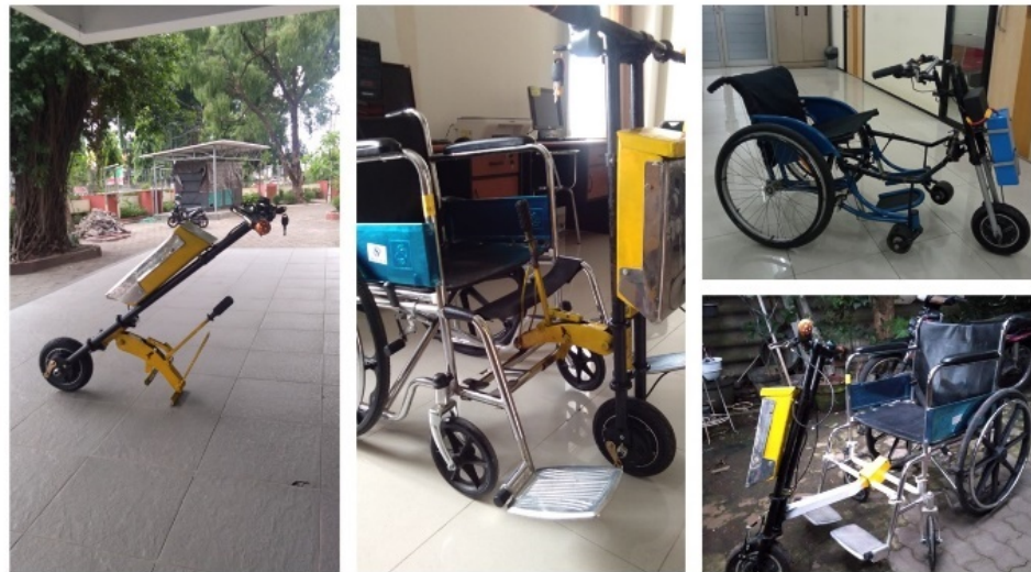
Figure 6: Model of detachable drive unit. Source: Adhitia Guspara et al. [20].
