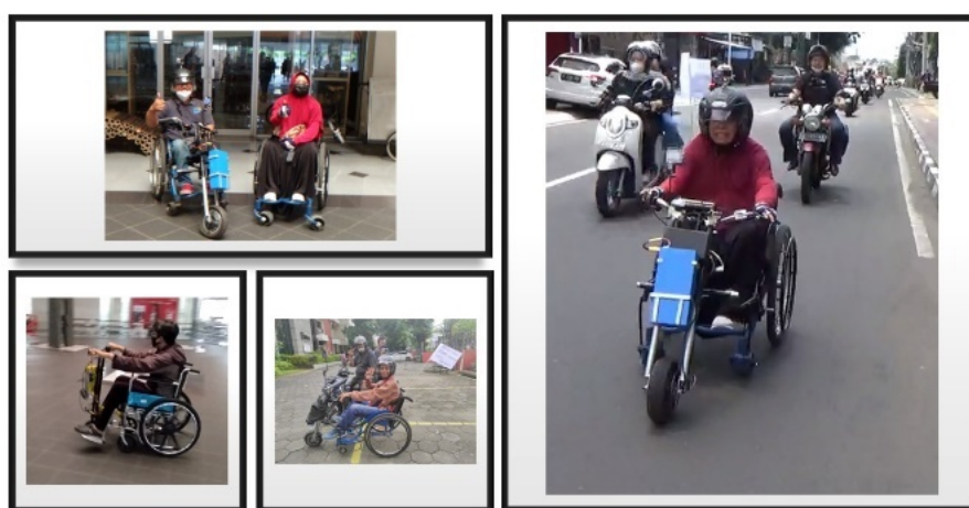
Figure 7: Fit testing detachable drive unit. Source: Research documentation, 2023.
