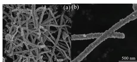
**Figure 2:** SEM images of NiO-SnO<sub>2</sub> nanofibers (a) with low magnification and (b) with high magnification.
