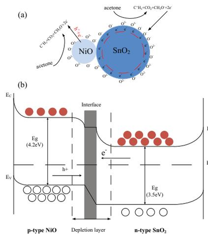
**Figure 5:** (a) Schematic model for the p-type NiO/n-type SnO<sub>2</sub> heterostructure based sensor when exposed to acetone. (b) Proposed band structure for p-type NiO/n-type SnO<sub>2</sub> heterostructure. E<sub>c</sub>: lower level of conduction band; E<sub>f</sub>: Fermi level; E<sub>v</sub>: upper level of valence band.
