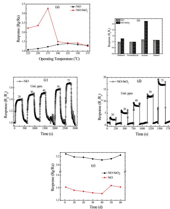
**Figure 4:** (a) Responses of the sensors based on NiO and NiO-SnO<sub>2</sub> nanofibers to 10 ppm acetone as a function of operating temperature. (b) Responses of NiO and NiO-SnO<sub>2</sub> to various gases including methanol, formaldehyde, acetone and ethanol. (c)(d) Dynamic sensing response of NiO and NiO-SnO<sub>2</sub> to acetone in a range of 20-75 ppm. (e) Stability of NiO and NiO-SnO<sub>2</sub> to 20 ppm acetone.
