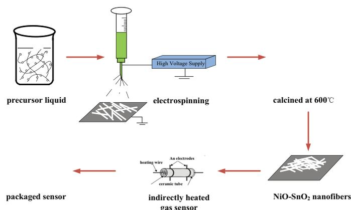
**Figure 1:** Schematic of the fabrication process of NiO-SnO<sub>2</sub> composite nanofibers based gas sensors.
