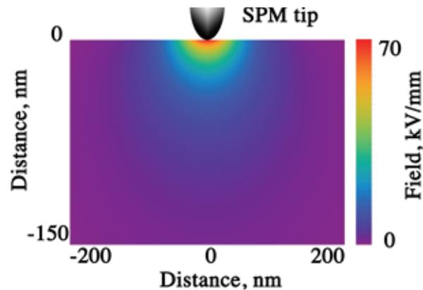
**Figure 1:** The calculated ZX distribution of the field, produced by SPM tip in contact with the polar surface of SBN61 ( $\epsilon_c = 900$ ,  $\epsilon_a = 450$ ,  $r_{tip} = 25$  nm,  $U_{sw} = 100$  V).
