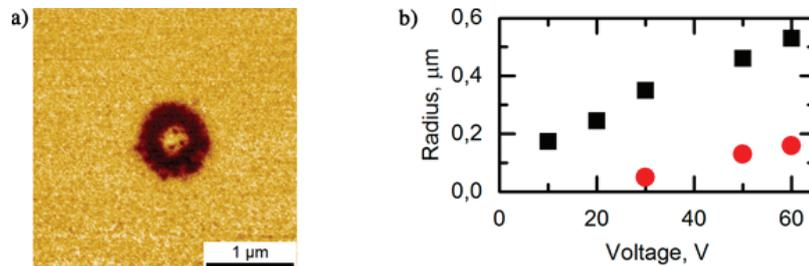
**Figure 7:** Backswitching of the domain formed by application dc voltage without tip withdrawal in SBN61:Ce in single domain state: (a) domain shape for  $U_{sw} = 50$  V and  $t_{sw} = 1$  s; (b) voltage dependence of the averaged domain radius for  $U_{sw} = 100$  V and  $t_{sw} = 32$  s (black squares) and averaged radius of backswitched domain (red circles).
