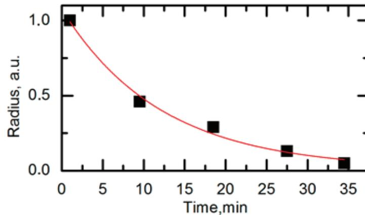
**Figure 6:** Relaxation of the radius of domain formed in SBN61:Ni in single domain state by dc voltage pulse with tip withdrawal.  $U_{sw} = 100$  V,  $t_{sw} = 1$  s. Experimental points fitted by exponential decay.
