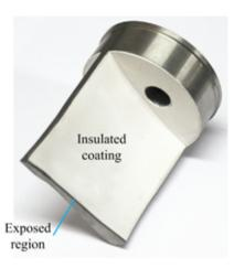
Figure 7: Result of designed cathode.
