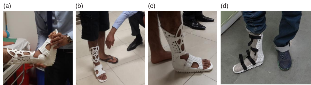
Figure 5: (A), Cast being tested on patient. (B), Cast tested with foot loading. (C), Cast tested for floor grip. (D), Walking Gait Testing with velcro band holding the foot.
