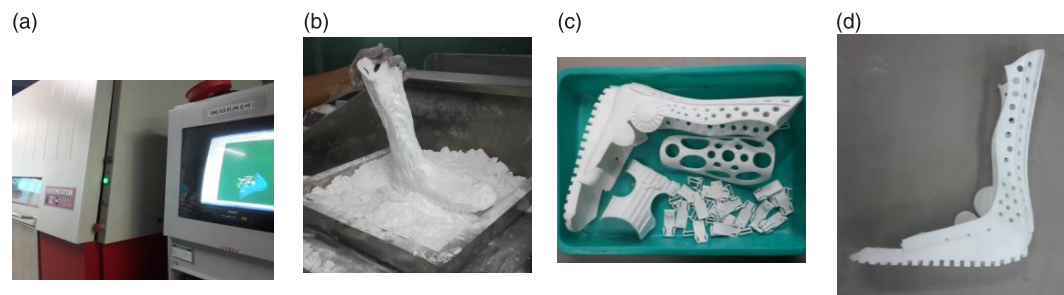
Figure 4: (A), SLS machine used to build the part. (B), Part being removed from the powder cake. (C), Nylon Parts made in SLS. (D), The bottom part of the cast.
