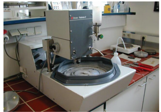
Figure 4: The polishing machine for ceramography. It is completed with upper and bottom disc to provide pressure during grinding and polishing.
