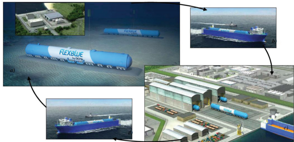
Figure 1: Artist views of a FLEXBLUE® module lifecycle: a) the subsea production site and the onshore control center; b) the ship transport; c) the support facility for refueling and maintenance; d) the transport back to the production site.
