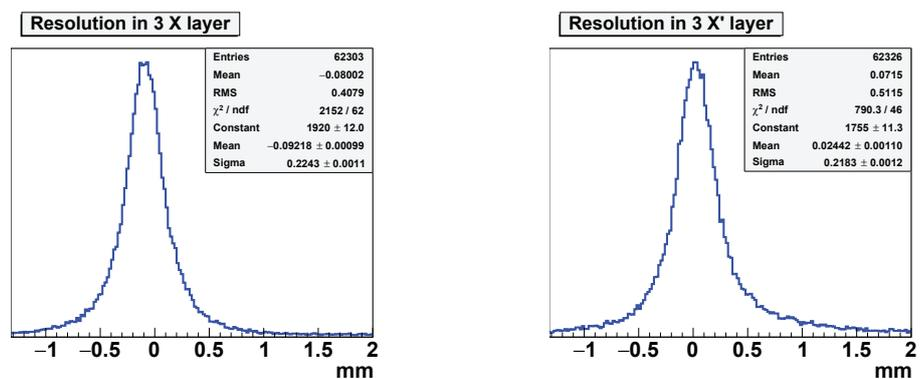
Figure 5: GEM Chamber 3 X and X' resolution with data for Ar+CO<sub>2</sub> gas mixture
