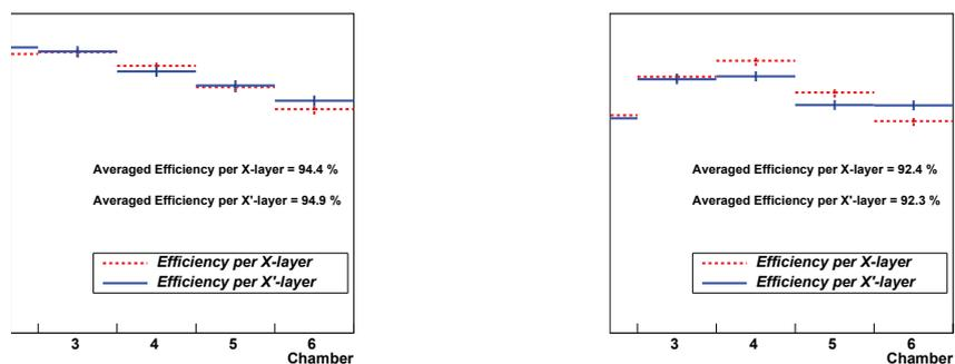
**Figure 3:** Efficiency per layer with Nuclotron data for two gas mixtures: Ar+CO<sub>2</sub> (left) and Ar+Isobutane (right)
