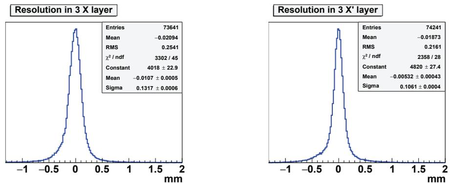
Figure 6: GEM Chamber 3 X and X' resolution with data for Ar+Isobutane gas mixture
