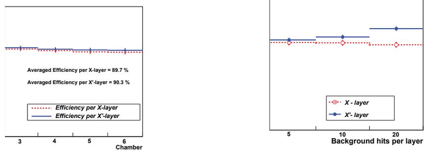
**Figure 2:** Calculated efficiency per layer (left) and dependence of efficiency vs background hits per layer (right) with Monte-Carlo data
