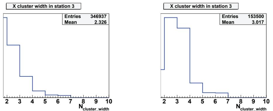
Figure 4: Cluster width for two gas mixtures: Ar+CO<sub>2</sub> (left) and Ar+Isobutane (right)
