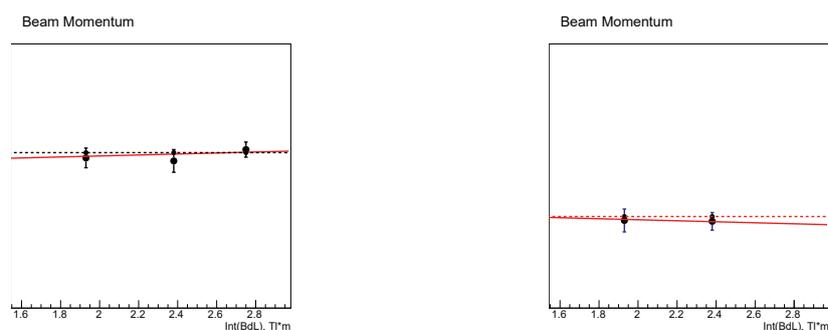
**Figure 1:** Two beam energy values: 4.5 GeV/nucleon (left) and 3.5 GeV/nucleon (right). The expected beam momentum value is indicated by dotted lines. Solid lines are experimental data.
