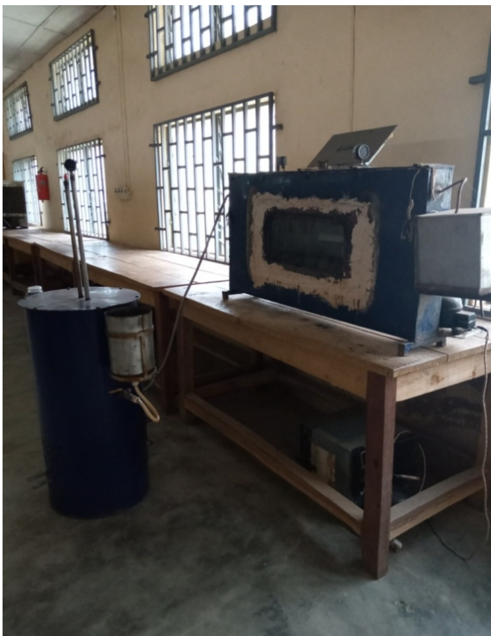
Figure 3: Steam Boiler, SandBox, and Condenser Set-Up.
